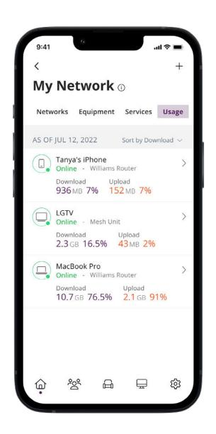
Network Usage is organized by device. From this view, you can see basic information about usage from each Wi-Fi connected device on your network, including: 1. Device identification and whether the device is connected 2. What network device it is connected to 3. Network usage 4. The amount of data that has been used by this device Network usage is updated each time you run a bandwidth test through the app.
