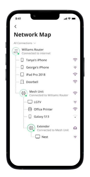
From the dashboard, you can select "My Network". This will show any GigaSpire BLAST or GigaMesh units connected in your network. Next tap into your Wi-Fi network from the Networks tab. From here, tap into the "Map" section to view devices connected to your system. You can tap on the Mesh icon to get performance information and devices connected at that Mesh unit.
