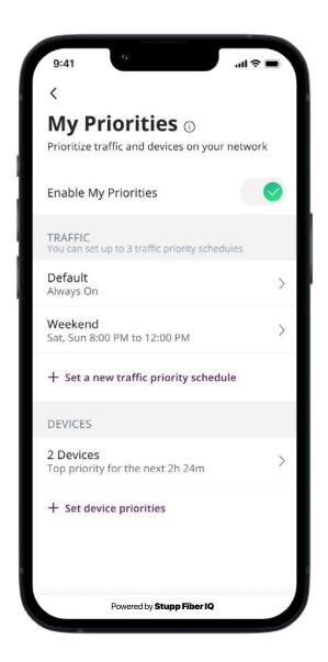
From any profile on the "Things" tab, tap into a device to access Network Priority to view activity and device prioritization settings.
